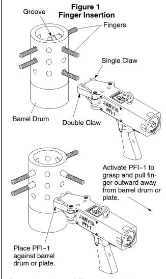
Figure above depicts PFI-1 with barrel drum containing round fingers. The PFI-1 can also be used for plates and rectangular fingers. **Note:** Rectangular fingers can only be installed one way. Check holes for proper orientation.
