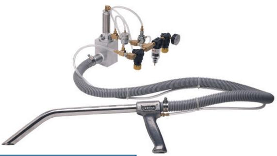
The Jarvis Model LKE-1 - pneumatically controlled gun for high speed vacuum removal of poultry lungs and kidneys.
